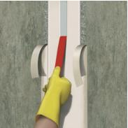
The adhesive top layer may be smoothed with a brush using a diluted detergent. Allow adhesive to start curing first.
