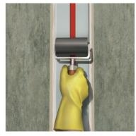
For fixing overhead or in difficult configurations, the tape may be temporarily held in place with Sika® Trocal Adhesive C-705. This adhesive, however may only be used in the tape centre but never on the areas to be bonded with Sikadur-Combiflex® CF Adhesive, Sikadur®-31 CF or Sikadur®-31 DW.
