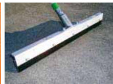
Sealing of a broadcast layer with a straight trowel or "squeegee" blade.
